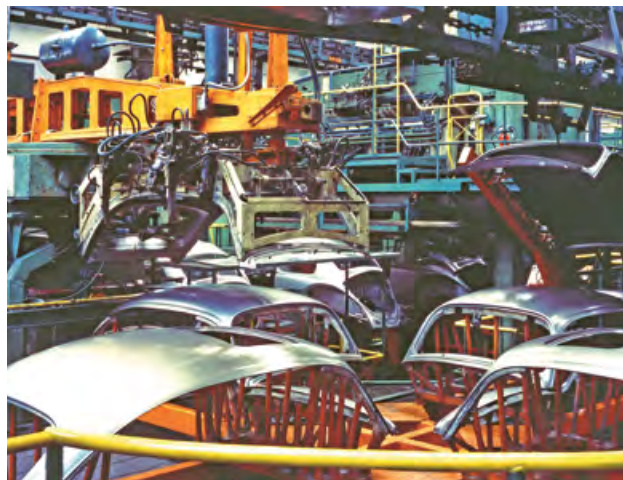
A KEY AUTOMATION STEP: THE TRANSFER LINE
