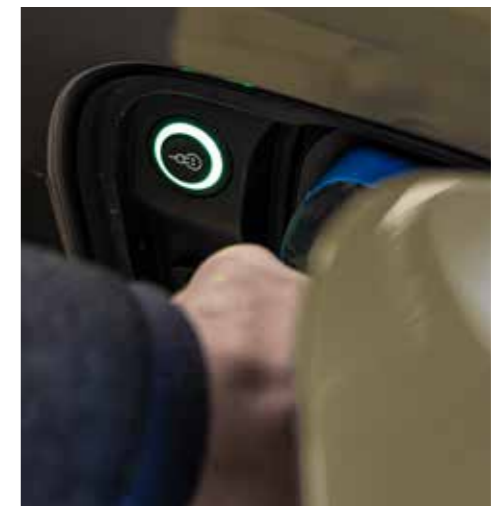
Good news for drivers of an Audi RS e-tron GT: 1 Thanks to its 800-volt technology, the high-voltage battery with 84 kWh of net capacity can be recharged extremely quickly.
