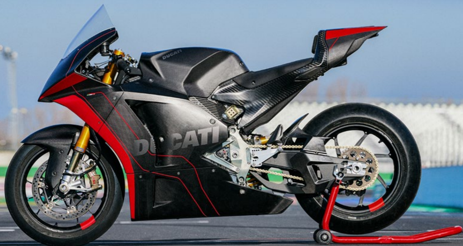
Ducati V21L, 1 electric prototype for the FIM (Fédération Internationale de Motocyclisme) Enel MotoE™ World Cup.
