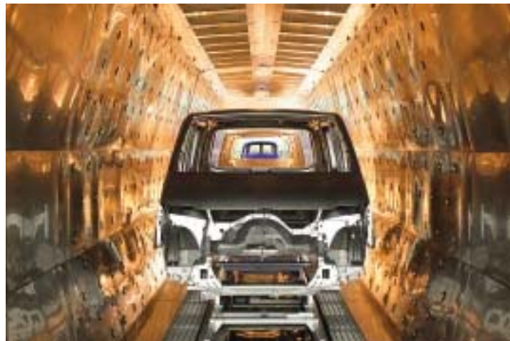
Color by color, the body shells make their way through the painting line.
