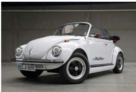
The e-Beetle – developed using electric components from the new e-up!
