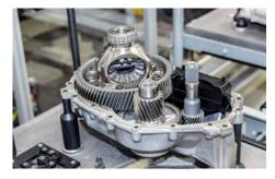
Small shifting unit: the 1-speed gearbox
